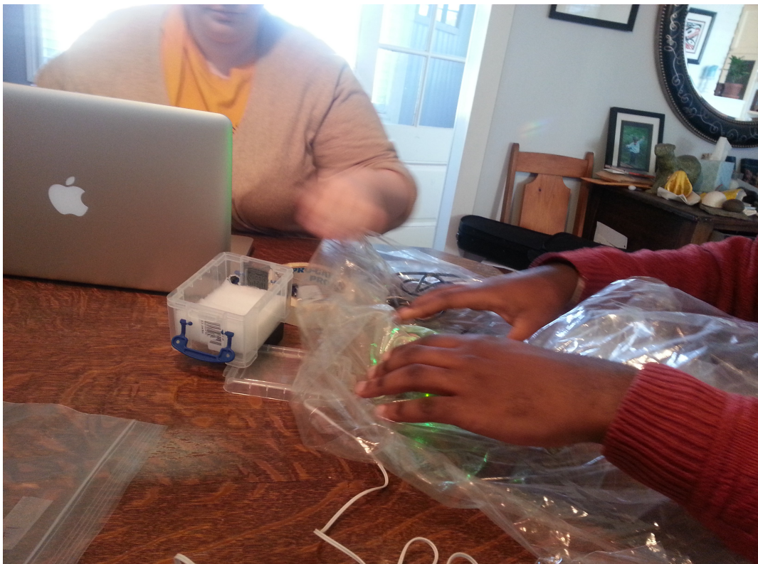
Checking temperature readings with and without plastics covering the sensor
