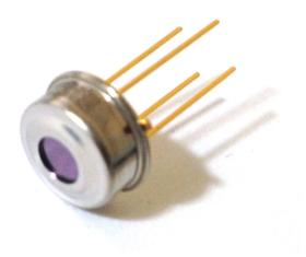
The MLX90614 is a sensor that can tell the temperature of something without touching it. By reading the infrared light coming off an object, the sensor can sense between -95 and 720°f (-70 to 382.2°C) with 17bit resolution. That degree of precision means it can tell the difference between 25°C and 25.02°C without coming in contact. (ie, 17bits should give us about 0.0034°C resolution).
