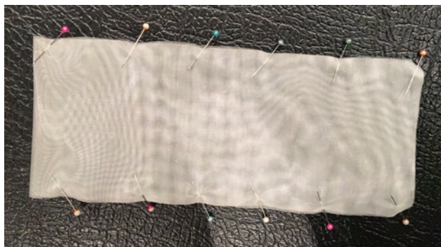
Figure 41: Step 5: Pin the cod end into shape to prepare for sewing.
