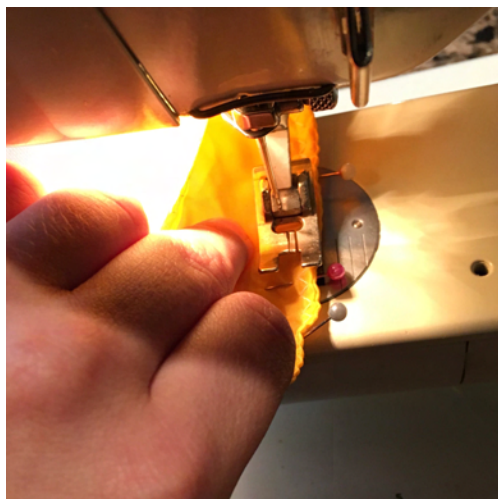
Figure 35: Step 16: Sewing the nylon reinforcement to the net opening.
