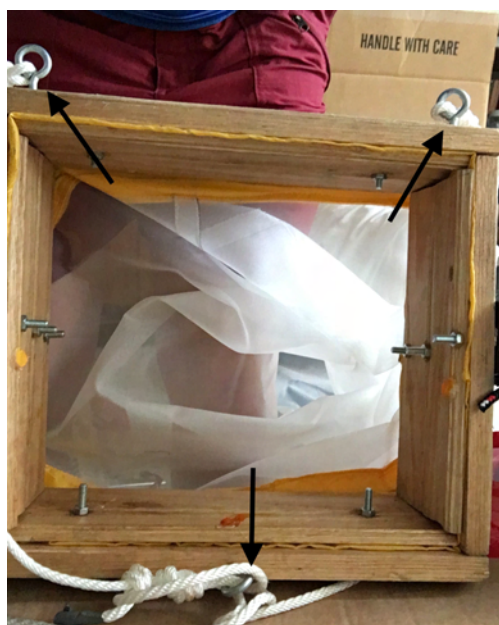
Figure 14: Step 15: Locations of the eyes used for trawling ropes
