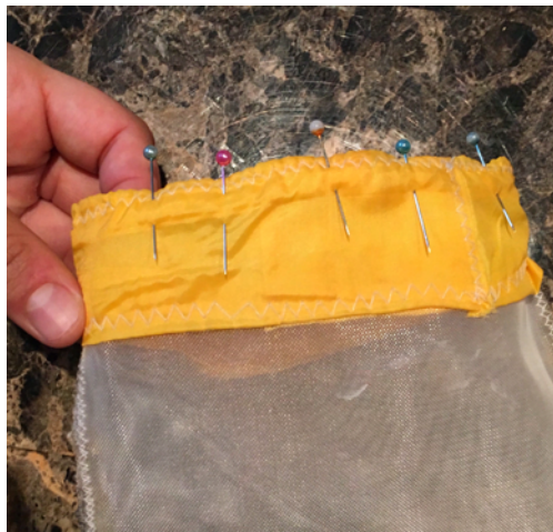
Figure 34: Step 15: Pinning the top edge of the nylon reinforcement to the net's openings.
