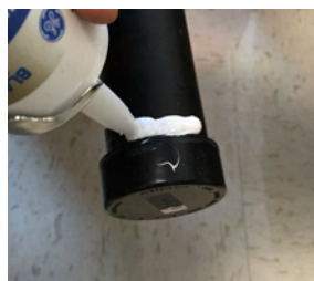
(a) Applying cement to the inner PVC and (b) Securing the pipe to the frame with a twist
