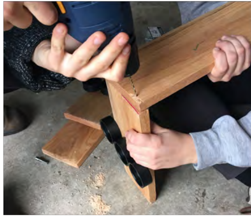
Figure 11: Step 3: Drilling pilot holes for woodscrews.
