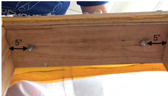
(a) Top of the frame, viewed from the inside (image not to scale. 5” is correct.)
