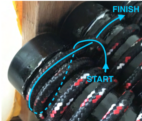
(a) A simple knot to anchor the rope
