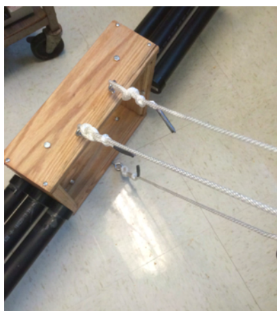
(a) Note: the trawling eyes are not placed properly in this picture, they should be 2" from the left and right edges.
