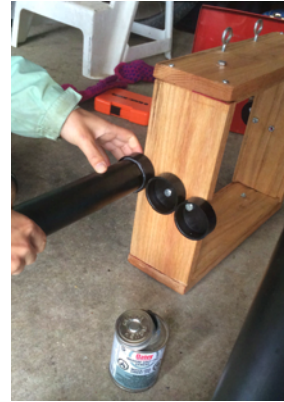
(a) Applying cement to the pontoons and (b) Securing the pipe to the frame with a twist.
