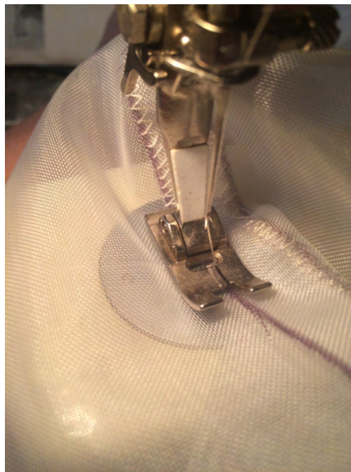
Figure 33: Step 13: The 'double seam' method for sewing a creaseless net.
