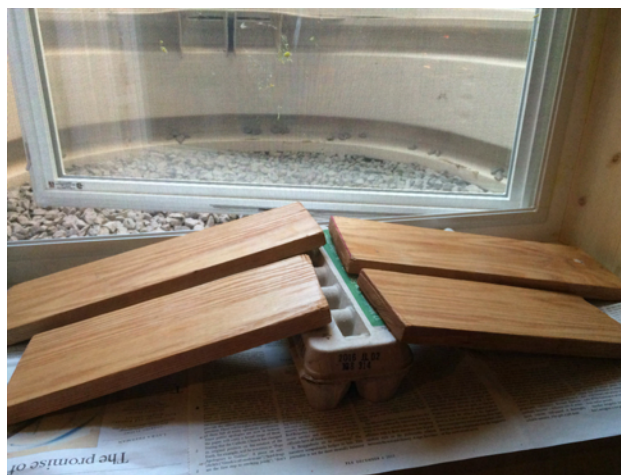
Figure 10: Step 2: Drying a coat of waterproofing on the oak frame pieces.
