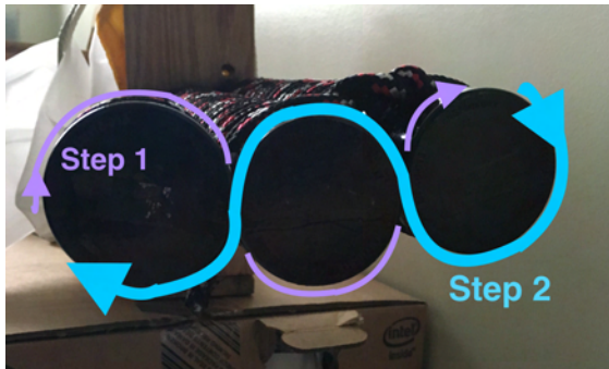
(c) The method of weaving the ropes between the PVC of the wings. Be sure to pull it tight at every of the ropes step for a snug fit!
