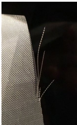
Figure 40: Step 4: Fraying edges can contaminate or lose samples.
