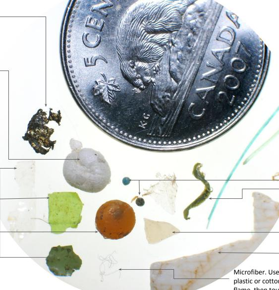
Thread plastic; thin with no cellular texture; frays are even (nylon rope)
