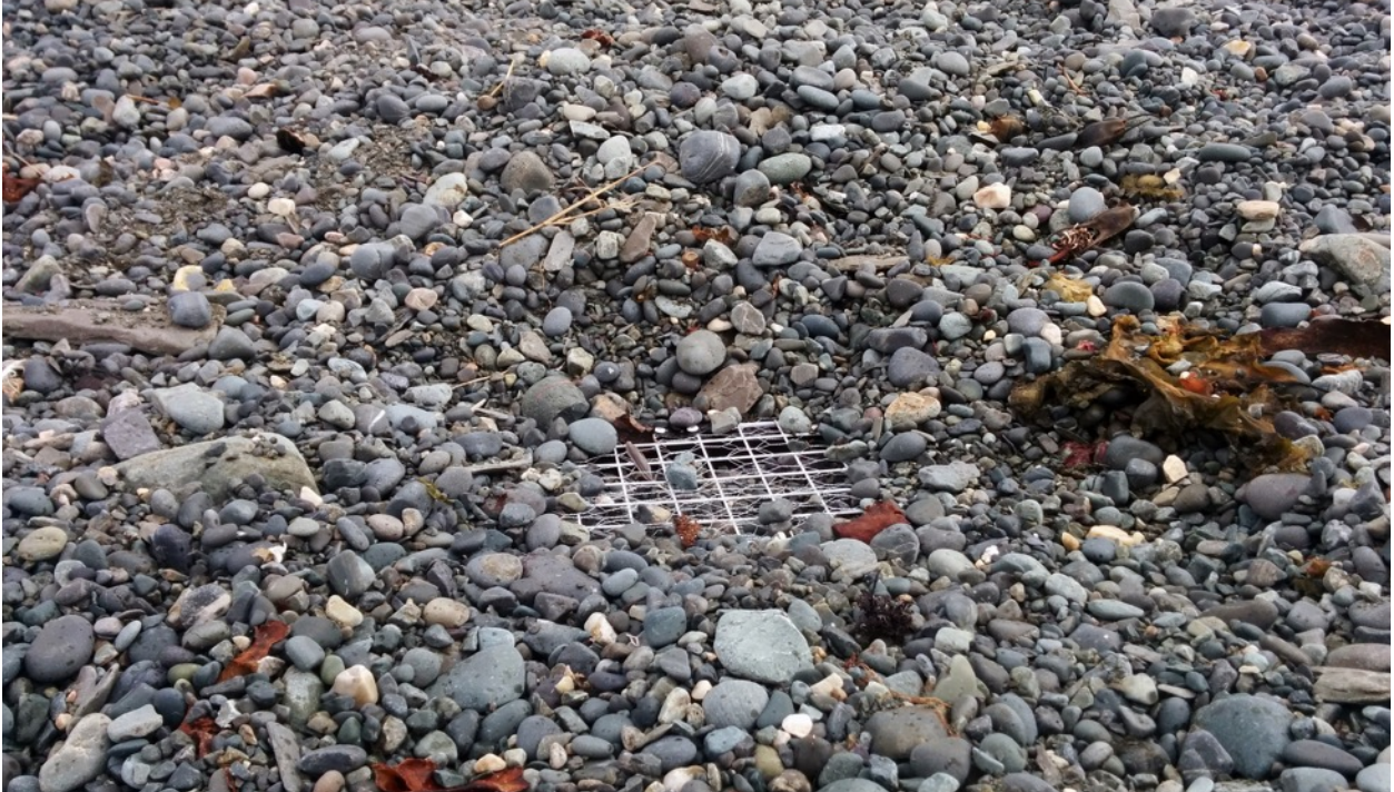
Figure 12 (above): Covering the PED ROC with a thin layer of rocks at the end. Many of these rocks will cover the device even more during wave action, so be sure to indicate where you've buried the device! We found that flags and lines were often buried, so we recommend triangulating landmarks and/or using GIS.
