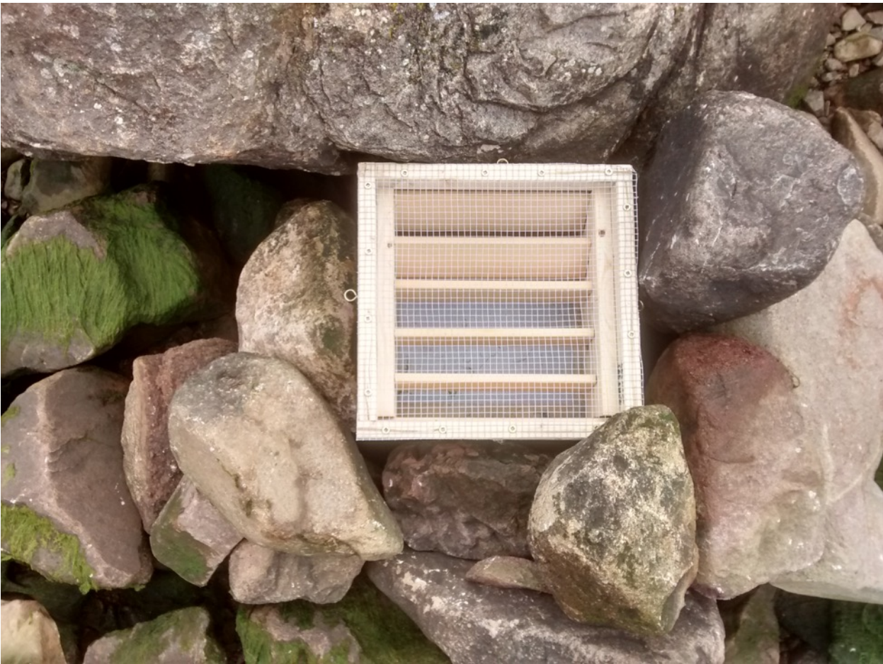
Figure 6 P.E.D. R.O.C. 2.0 with wooden slats that closed when water rose. The problem with this design is that the wood could swell. Summer 2015.
