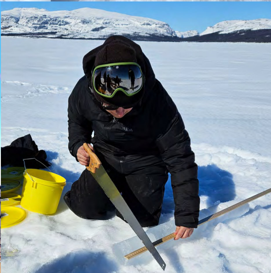
Top left: Liz Pijogge shows Mannasse (sp) Pijogge and Paul McCarney how to work the ice corer. Top right: Liz displays an ice core. Bottom left: Liz drills holes in each core section to take their temperature. Photos: Max Liboiron. Bottom right: Max Liboiron measures and cuts the core into sections. April 2024. Photo: Liz Pijogge
