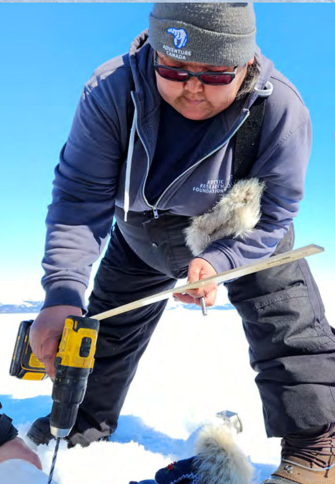
Top left: Liz Pijogge shows Mannasse (sp) Pijogge and Paul McCarney how to work the ice corer. Top right: Liz displays an ice core. Bottom left: Liz drills holes in each core section to take their temperature. Photos: Max Liboiron. Bottom right: Max Liboiron measures and cuts the core into sections. April 2024. Photo: Liz Pijogge
